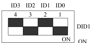
The above chart shows "0101", so it means that the physical ID is 5.
